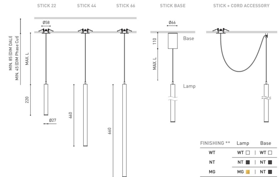
BASE NOT USED WITH WIRE TRIMLESS INSTALLATION.
